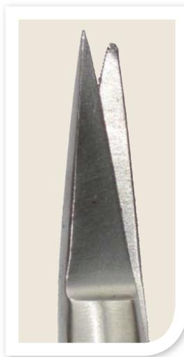
Scissors (and all other hinged instruments) must be cleaned and sterilised frequently. When the scissors are cleaned with the blades in a "closed" position the blades (which are the most sensitive part) are under light pressure. Due to the heat of the autoclave the metal expands, which increases this pressure. The points may be affected by this pressure and breakage could occur.
