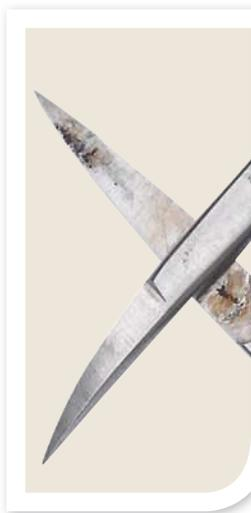
High grade stainless steel is stain "less" but is not immune from corrosion. At the pivot of the hinge friction occurs. The particles produced by this friction come into contact with oxygen and water and the rust process starts. During sterilisation transference of rust can be transmitted to and attack the metal of other instruments. "Transferred rust" is found mainly in areas of the hinge and the blades, as these areas
